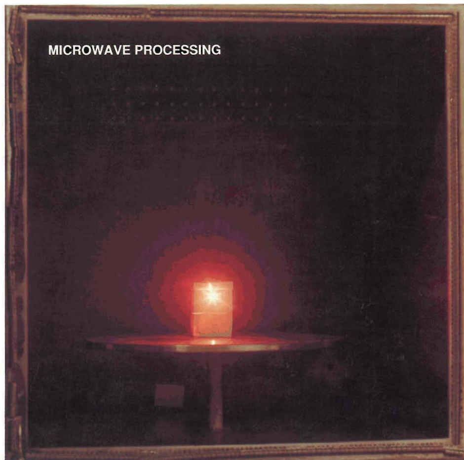
Fig. 11. A sample of boron carbide is rapidly sintered in a microwave oven to produce a fine-grained ceramic with a density that is close to the theoretical maximum.
