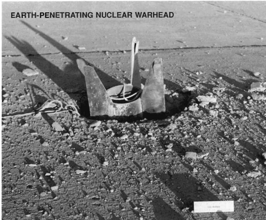
Fig. 3. Test photographs of a warhead designed to penetrate the ground before detonating. In this particular test the warhead penetrated a foot of concrete over hard dirt and came to rest almost nine feet below the top surface. In subsequent tests, an improved warhead penetrated the concrete completely.
